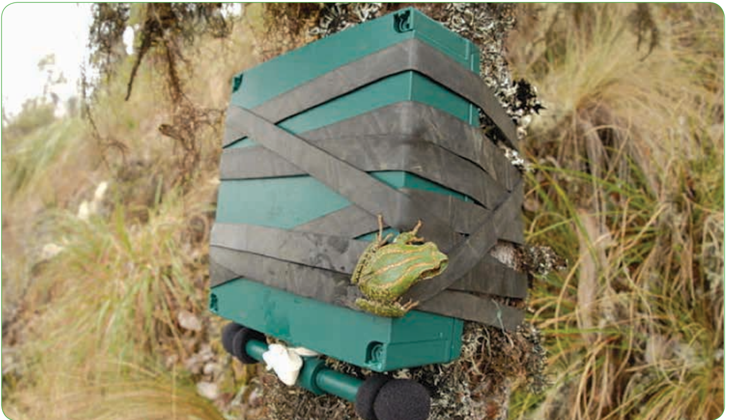
Figure 1 Automatic digital sound recorder used to monitor populations of marsupial frogs ( Gastrotheca excubitor in the image) and terrestrial breeding frogs ( Noblella pygmaea and Psychrophrynella usurpator ) at the Abra Acjanaco mountain pass in the Peruvian Andes (photo by A. Catenazzi).
