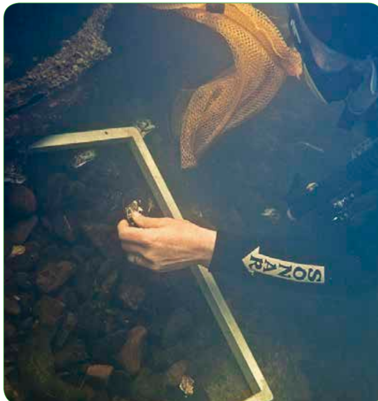
Figure 13 A quadrat frame used to conduct quantitative surveys for freshwater mussels and large gastropods.
