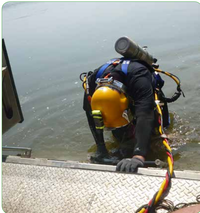
Figure 11 A diver, using surface supplied air commonly referred to as a “Hookah rig”, to sample in large, deep rivers. Mississippi River, Illinois, USA.
